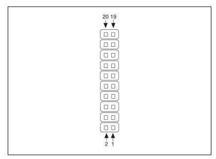
Figure B-12. Front Panel Connector (JF1)
